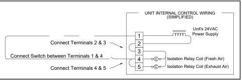
FIGURE 5.6.0 SINGLE 2-WIRE CONTROL, UNPOWERED
