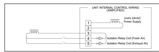
FIGURE 5.6.4 CONTROL WITH 2 "ON" SIGNALS, EXTERNAL POWER
