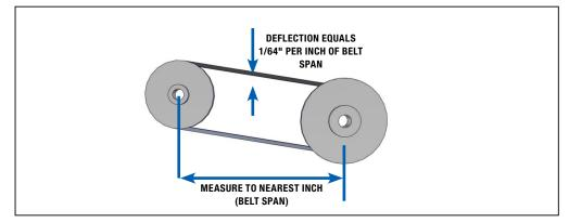
FIGURE 7.5.0 FAN BELT TENSIONING
