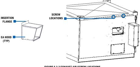
FIGURE 5.3.2 EXHAUST AIR SCREW LOCATIONS
