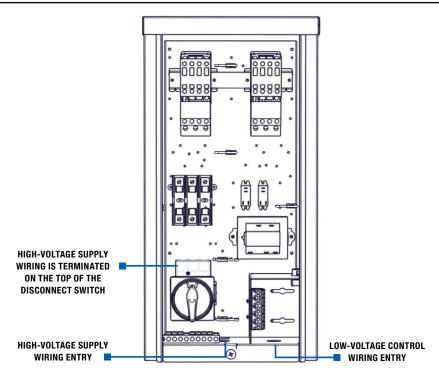
FIGURE 5.4.0 E-BOX WIRING ENTRY POINTS
