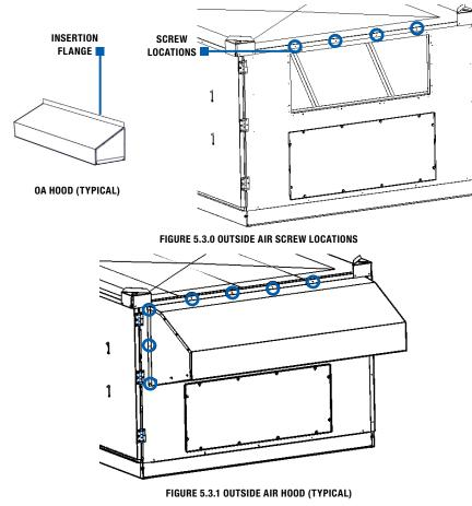
Slip the top flange of the OA hood assembly under the roof panel overhang to flash the hood assembly from precipitation. You may need to pry the roof panel overhang away from the unit side pan to get the hood assembly top flange under that roof panel overhang. Align the side screw holes on the hood assembly with the holes in the unit side pan and attach the hood assembly with screws (provided). Replace the self-tapping screws that were removed from the roof panel overhang above the hood.
