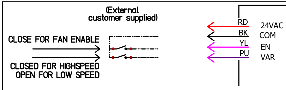
FIGURE 5.6.0 FIELD CIRCUIT DETAIL
