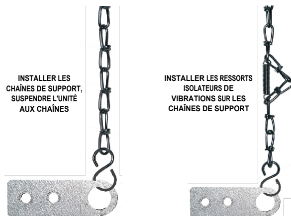
FIGURE 2.1.3 INSTALLATION DES CHÂÎNES DE SUPPORT
